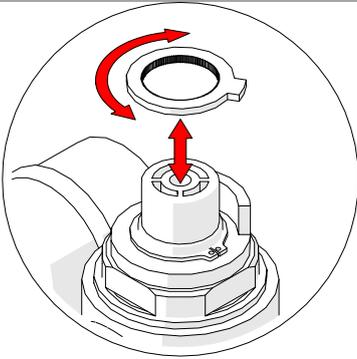
4. Remove the lower brass ring (temperature setting ring) and rotate the brass ring clockwise to increase temperature or anti-clockwise to decrease.
